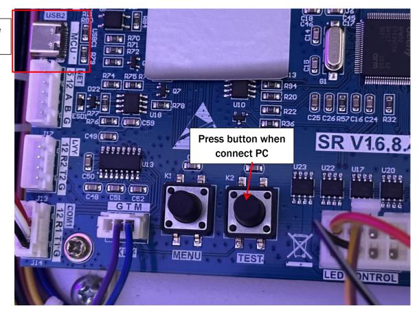
Step 4 Locate PC. Select "打开固件"(Open Software). Select latest software(Bin. format). Note: Picture software is only for reference.
