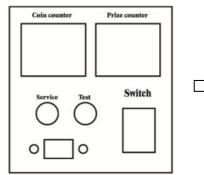
Open the coin door and there is a meter panel. Long press Service button for 5 seconds to enter the setting menu.
