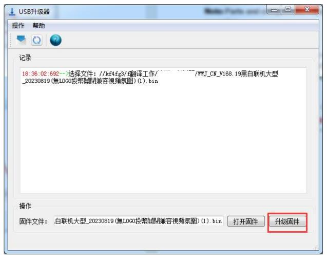
Step 6 When you see " (Success)", Update finish! Unplug the mainboard. Step 7 Install Mainboard back to the machine. Power on the machine.
