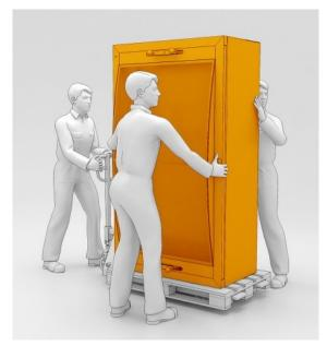
When transporting the packed machine, it is suggested that the device be secured by 2 people as shown in the picture.
