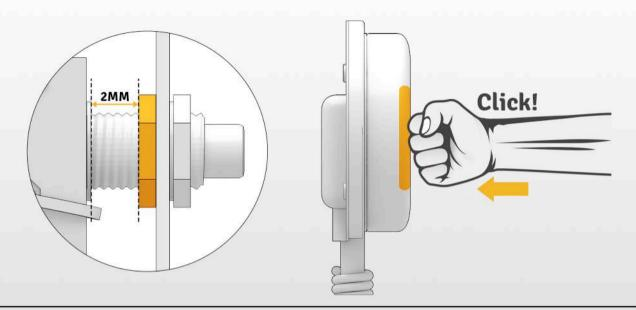
The sensor is moved to the direction shown in the picture by about 2mm.
